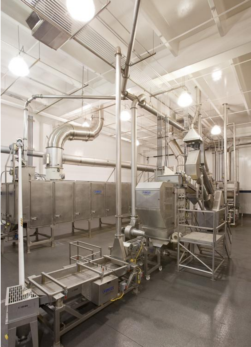
LOST HILLS, Calif., November 2, 2009 – Paramount Farms' new almond manufacturing plant's design minimizes contamination. The concrete structure is built without exposed beams, seams or sub-walls for durability and contaminant control while a HEPA air filtration system helps remove potential foreign airborne particles.
